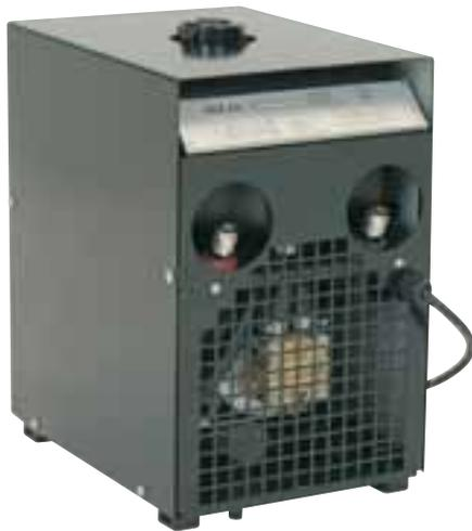
The OCE-2 H water-cooling unit is an efficient, compactly-dimensioned cooling unit designed for use together with water-cooled equipment for arc welding by hand or in automatic plants. The water tank and pump is made of corrosion-resistant material.
